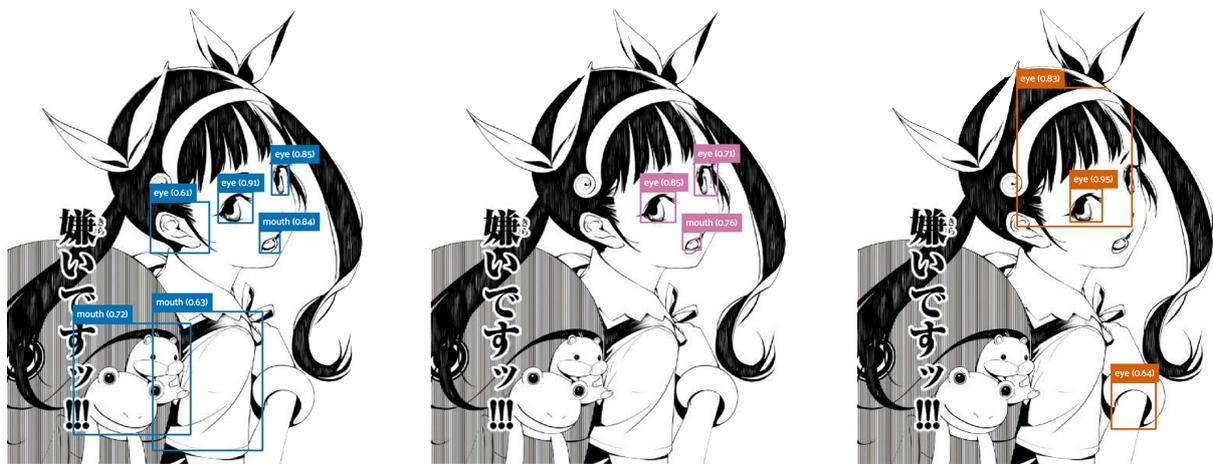
**Figure 1: Eyes and Mouths Detected by Our Three Fine-Tuned Models.** From left to right, the images show inferences from our three trained models: YOLOX-L, YOLOX-Tiny, and Faster R-CNN. YOLOX-Tiny outperforms the other two, while YOLOX-L produces false positives, and Faster R-CNN fails to detect correctly.
